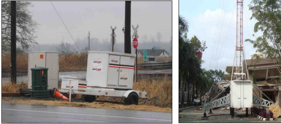
Figure 38. Switch on wheels (left) and cellular on wheels (right) (Photograph taken by A. Tang, L & T Consulting).
