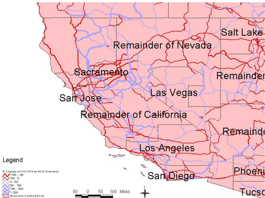
Figure 66. National highway network volume change for northern California storm on day 14.
